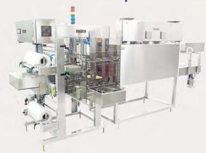
Autopack SLC with welding bar is a medium speed Bundle Shrink Wrapper equipped with cardboard pad inserter. Side infeed can be single lane infeed with horizontal collator with collation done directly onto the pad. For higher speed line, the machine can be configured with multilane infeed also directly onto the pad. The use of cardboard pad gives extra strength to shrink wrapped products for better handling and stability on pallet for a minimum cost of cardboard.
