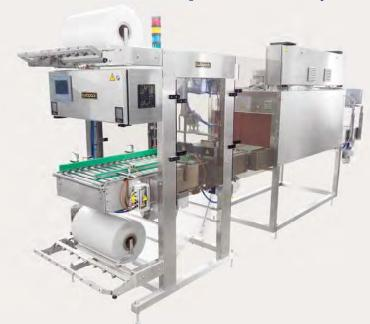
Autopack SIT with welding bar is a medium speed Bundle Shrink Wrapper designed to handle pre-loaded trays, single boxes or stacked rigid items. The inline design combined with Autopack compact footprint wrapper and tunnel facilitate economical use of valuable factory space.
