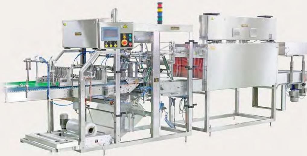
Autopack SIM CMOS is a Continuous Motion Overlap Seal bundle shrink wrapper with Inline Infeed on Multiple lanes, designed for handling all product types that can be accumulated (i.e. bottles, cans, cartons) from all industry sectors. With a maximum speed of 45 cycles/min, it is Autopack's fastest machine and among the world's most compact overlap seal machines with speed up to 135 packs/min (triple tracks).
